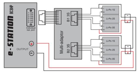
ex) 3 x 2S connection using serial charging
