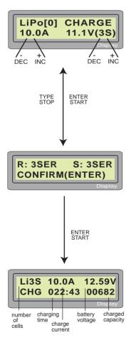
The left side of the first line shows the type of battery and data number. The value on the left side of second line sets a charge current and the value on the right side sets the voltage of the battery pack. In 'AUTO', the charger will check the cell-count of battery automatically.
