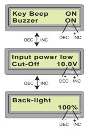
The beep sounds at every time pressing the buttons to confirm your action. The beep or melody sounded at various times during operation to alert different mode changes. These audible sounds can be on or off.
