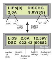
The value of discharge current on the left side of screen may not exceed 1C for a maximum safety. The final voltage at the end of discharge is on the right according to the cell count and type of battery. For LiPo, it is 3.0V/cell.
