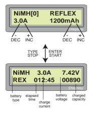
The battery will be charged using the pulsed current which is very brief and high-rate discharge pulses. This will help to prevent from undesired side effect like 'memory effect'. When you select this mode, you need to set the partial capacity which will be charged with reflex mode. The charger will work with 'Reflex' mode only until the capacity has been charged, then the charger will work at 'Normal mode'.
