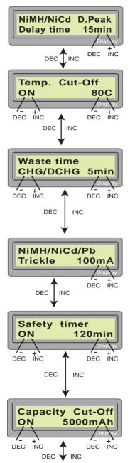
This restrains the delta-peak voltage detection until the time has reached. This prevents a premature cut-off from the battery of high internal resistance. The default value is one minute.  $(1 \sim 15 \text{ minutes})$
