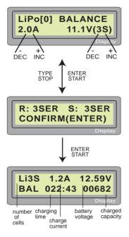
The value on the left side of second line sets a charge current and the value on the right side of second line sets the voltage of the battery pack.
