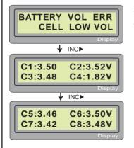
The processor found that the voltage of one of the cell in the Lithium battery pack is too low.
