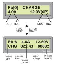
Set up the charge current on the left and the nominal voltage of the battery on the right. The charge current ranges from 0.1 to 12.0A and the voltage should be matched with the battery being charged.
