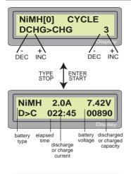
Set the sequence on the left and the number of cycle on the right. You can use this function for balancing, refreshing and break-in the battery. To avoid rising temperature of the battery, there will a brief cool-off period that already fixed at 'User program setup' after each charge and discharge process.
