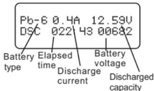
The screen display the real-time discharging status. Press START/ENTER button to change the discharging value. Press START/ENTER button again to store the parameter value you set. Press BATT TYPE/STOP button to end the program.
