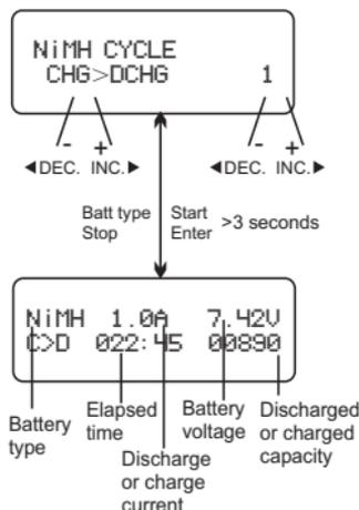
You can set up sequence on the left and the number of cycles on the right. Range of the cycle number is 1-5.
