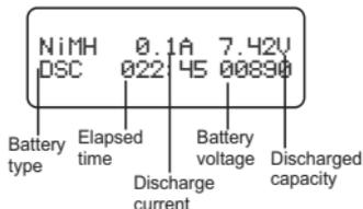
The screen indicates the discharging state. you can press START/ENTER button to alter discharge current, Press START/ENTER button again to store the value, Press BATT TYPE/STOP button to stop discharging. The emitted sound alerts the end of discharging.
