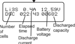
If both numbers are identical you can start charging process. If not, press BATT TYPE /STOP button to go back to previous screen to recheck the number of cells of the battery pack before going ahead.
