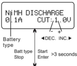
Set discharge current on the left and final voltage on the right.
