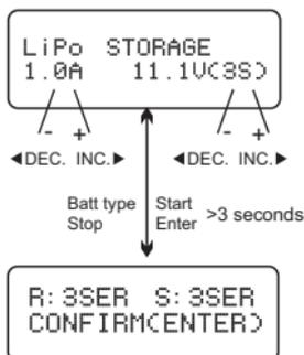
At this screen, you can set up the current and voltage of the battery pack. Charging and discharging will make the batteries come to the voltage level of storage state.
