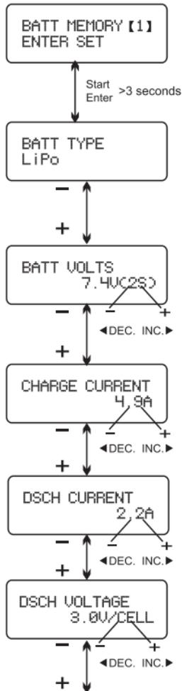
For your convenience UP200 Duo has a data storage and load program, it can store 10 different battery data represent the respective specifications of batteries, you can call back the data when charging/discharging without setting up the program again, press START/ENTER button to make it blink and use INC. or DEC. to set up the parameter.
