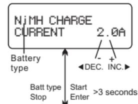
This program is for charging and discharging of NiMH/NiCD batteries associated with R/C models applications. You can press Inc. or Dec. button to change the parameter value, press START/ENTER button to store the value.
