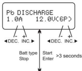
Set up the discharge current on the left and nominal voltage on the right. Range of discharge current is 0.1-5.0A the voltage should match the battery being discharged. Press ENTER/START button for more than 3 seconds to start discharging.
