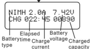
The screen displays the real-time charging status. Press BATT TYPE/STOP button to stop the process. The audible sound indicate the end of process.
