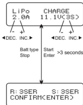
The left side of the first line shows the type of battery you choose. The value on the left of the second line of the charger is current the user sets. After setting the current and voltage, press the START/ENTER for more than 3 seconds to start the process.
