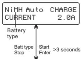
The program is for charging of NiMH/NiCD batteries in auto mode.
