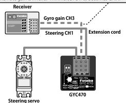
\* When using SR mode, SBUS connection is not possible. When using SR mode, connect as shown on the left.
