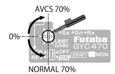
Receiver ON  $\rightarrow$  The GYC470 requires 3-5 seconds to initialize when the power is turned on. Do not move the car and do not move the steering wheel during this initialization or the gyro may not initialize properly. Once the initialization process has been completed, the steering servo will move slightly several times, indicating that the GYC470 is now ready for use. If neutral has shifted, LED will blink orange. In that case, it reboots.
